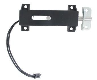
This sliding bolt security latch/switch is FMVSS 217 compliant for bus window emergency exits. It contains an integrated micro switch that is designed to actuate an audible signal to the driver when the slide latch is locked and the vehicle's ignition is in the "on" position
